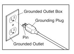
electric current to reduce the risk of electric shock. This product is equipped with a cord having an equipment-grounding conductor and a grounding plug. **Plug** the power cord into an appropriate outlet that is properly installed and grounded in accordance with all local codes and ordinances. This product is for use on a nominal 120-volt circuit. Important: The elliptical exerciser is not compatible with GFCI-equipped outlets.
